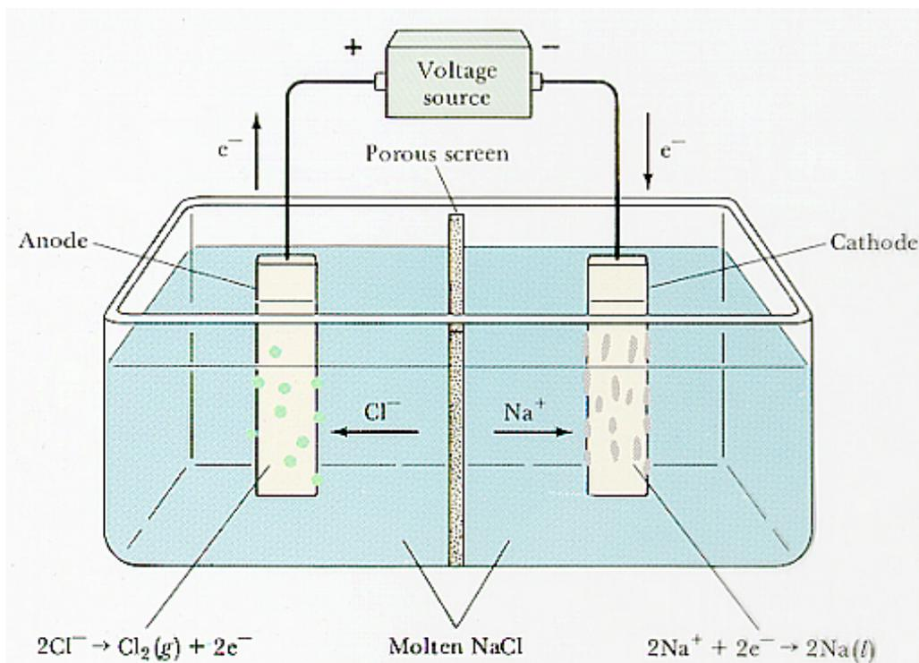
**Oxidisation of  $\text{Cl}^-$  taking place at Anode**
