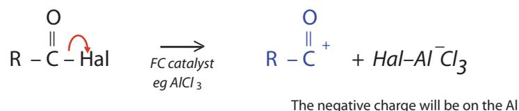
The common reaction mechanism for the **Halogenation** (replacing an H atom with an “Hal” species), **Alkylation** (replacing an H atom with a “ $C_nH_{2n+1}$ ” species), **Acylation** (replacing an H atom with an “ $R-C^+=O$ ” species) and the **Nitration** (replacing an H atom with a “ $NO_2^+$ ” species) of Benzene is
